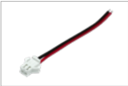
SM-2A male connector, 2 cores, UL2468 20AWG L=80/2mm
